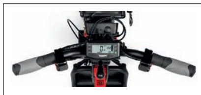
G&B handlebar option without levers for quadriplegics.
